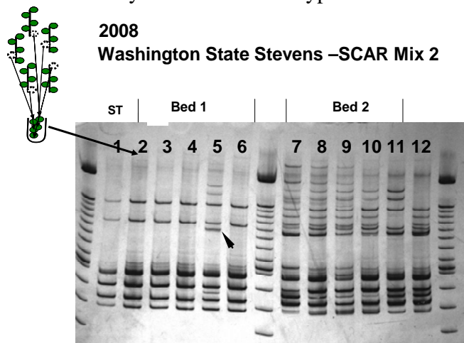
Fig. 2. Example of a gel with 12 samples. Lane 1 is our Stevens control. Lanes 2 – 6 represent 5 samples from 1 Stevens bed, and lanes 7-12 represent samples from a 2 nd bed. Note: lanes 2 – 4 and 6 match our Stevens control (lane 1), whereas lane 5 does not. It has some additional bands indicating there at least one subsample was not Stevens. Bed 2 (Lanes 7 – 12) has no match to Stevens, indicating considerable contamination. Arrow indicates extra non-Stevens bands in lane 5.
